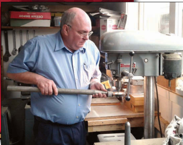
Pipe repair—cleaning debris off a reed pipe block
